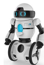
Fig. 1. This toy robot is an example of a single axle two wheeled robot, whose equations of motion can be used to plan its trajectory. This image was taken from https://www.ucsdrobotics.org/mips
